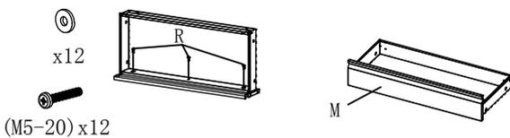
5. Place the assembled drawer attached to the cabinet, and adjust the spacing between the drawer and tighten R
